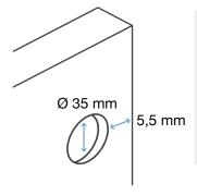
The hinge holes are set back by 5.5 mm as standard and have a diameter of 35 mm. If you want different measurements for the hinge hole, you can specify them in the configurator.
